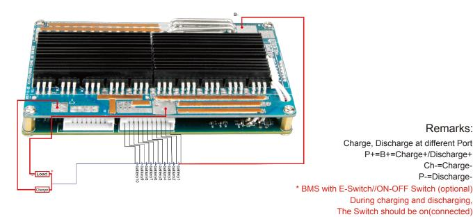
\* Note: The switch is not included, BMS has the E-Switch function. When the switch is off, the output will be shut down completely!
